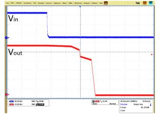
Shutdown by power-off (V<sub>in</sub> = 240 V DC, V<sub>out</sub> = 53.5 V DC)
