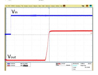
Startup by power-on (V<sub>in</sub> = 240 V DC, V<sub>out</sub> = 53.5 V DC)
