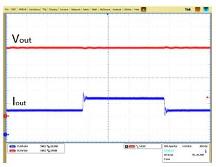
Output voltage dynamic response ( $V_{in} = 240 \text{ V DC}$ ; load: 50%–75%–50%; 1 A/µs; T = 4 ms;  $V_{out} = 53.5 \text{ V DC}$ )
