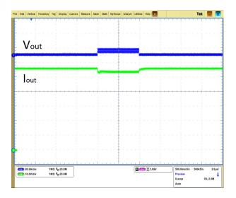
Output voltage dynamic response ( $V_{in}$  = 220 V AC; load: 25%–50%–25%; 1 A/µs; T = 4 ms;  $V_{out}$  = 53.5 V DC)
