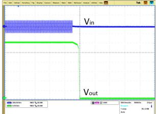
Shutdown by power-off (V<sub>in</sub> = 220 V AC, V<sub>out</sub> = 53.5 V DC)
