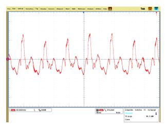
Output voltage ripple (V<sub>in</sub> = 240 V DC, V<sub>out</sub> = 53.5 V DC)
