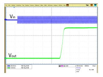
Startup by power-on (V<sub>in</sub> = 220 V AC, V<sub>out</sub> = 53.5 V DC)
